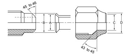
Fig. 3-2-2 Relations between flare nut and flare seal surface
