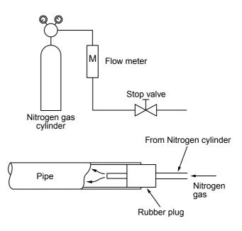
Fig. 3-5-1 Prevention of oxidation during brazing
