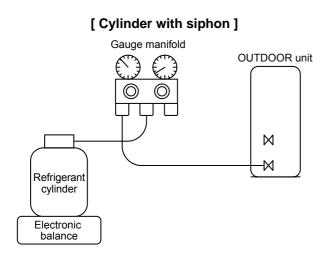
R410A refrigerant is HFC mixed refrigerant. Therefore, if it is charged with gas, the composition of the charged refrigerant changes and the characteristics of the equipment varies.
