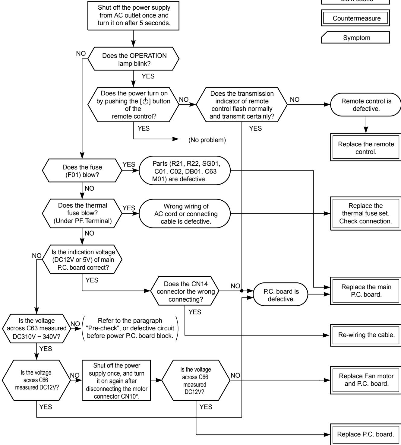
\* Be sure to disconnect the motor connector CN10 after shut off the power supply, or it will be a cause of damage of the motor.
