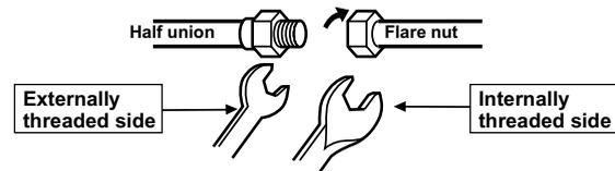
Use a wrench to secure. Use a torque wrench to tighten.
